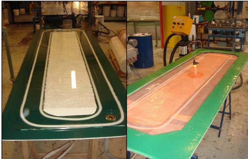
Fig. 1 RTM light / ECO and CCBM linear tool.
